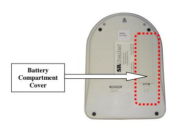
Figure 1: Battery Compartment Cover
