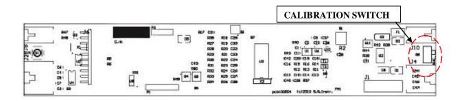
Figure 6: Calibration Switch Diagram
