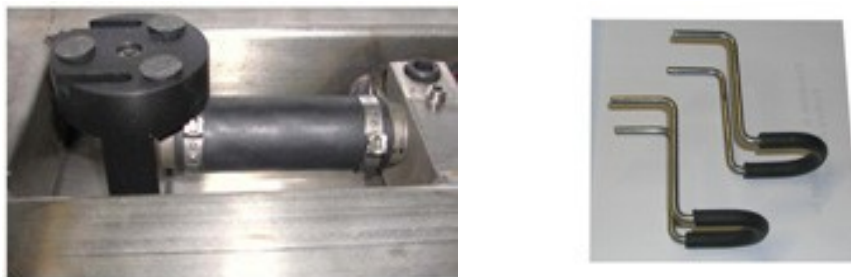
Figure 2: Load Cell Slots & Edge Anchors
