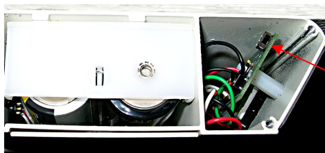
Figure 6: Display Board Calibration Switch Location
