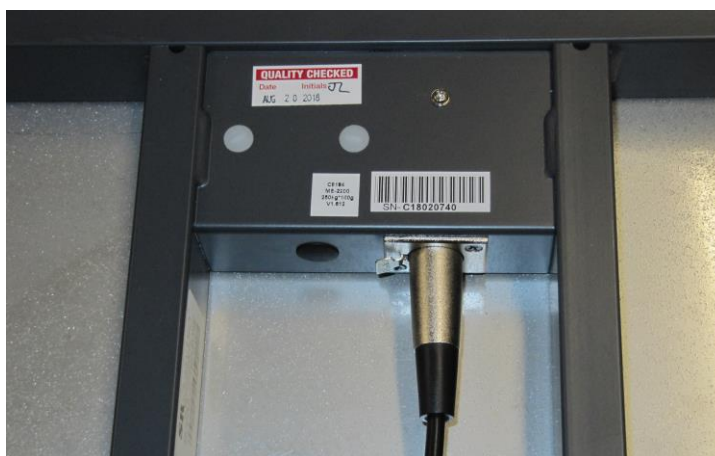
Figure 2: Cable Connection to Platform
